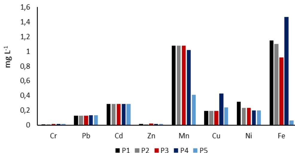
Figure 3: Contents of heavy metals analyzed as a function of sampling site.
