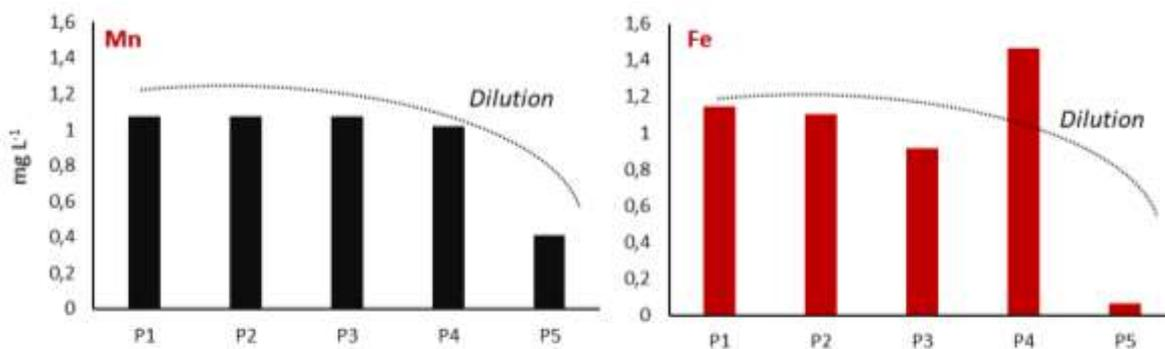
Figure 4: Phenomenon of the dilution of heavy metals at point P5, for manganese (A) and for iron (B).
